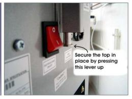
2. Once the top is installed and slid all of the way to the rear of the machine, engage the lock on the back to secure the top in place.
